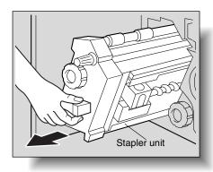
4 Grasp both sides of the staple cartridge holder, lift it up, and then pull it out.
